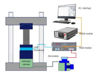
Test control scheme for Servohydraulic Compression Testing Machines.
