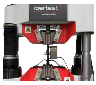
Tensile test of a cylindrical specimen. Deformation measurement through clamp exteensometer IB-MFA20
