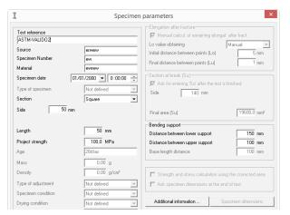
Setting parameters for the test specimen
