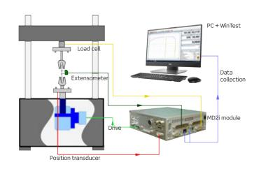
Test control scheme for Servohydraulic Universal Testing Machines.
