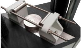
Bending testing device
