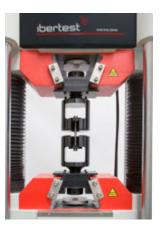
Accessory: tensile device for cabezales for button or/and threaded shoulded metallic specimens
