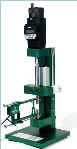
Model 3590 calibrator with Model 3542 axial extensometer
