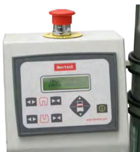
UCRB: Remote Control for opening/closing jaws and piston positioning
