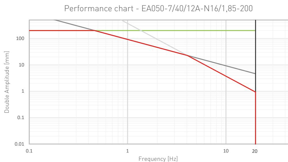
Stroke Limit    Speed limit    Acceleration limit    Frequency Limit    Total Performance
