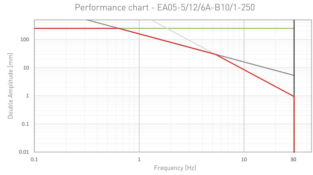
— Stroke Limit — Speed limit — Acceleration limit — Frequency Limit — Total Performance
