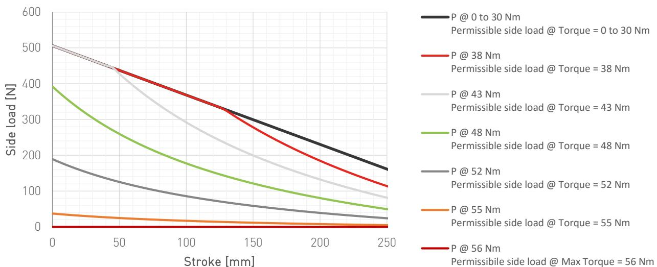
Permissible torque for a given side load
