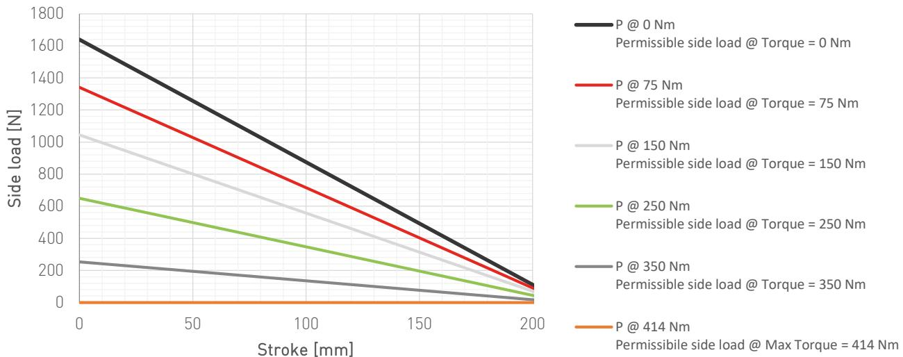
Permissible torque for a given side load
