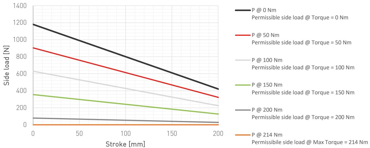
Permissible torque for a given side load
