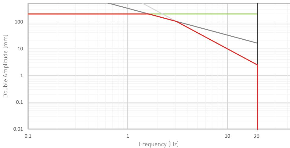
Stroke Limit    Speed limit    Acceleration limit    Frequency Limit    Total Performance
