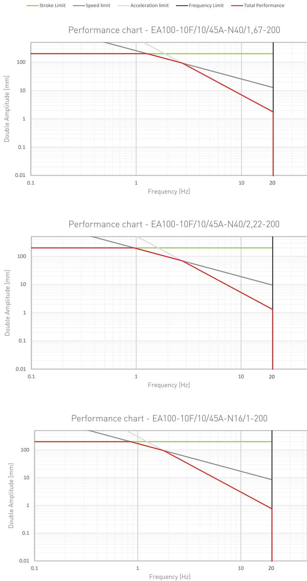
Stroke Limit    Speed limit    Acceleration limit    Frequency Limit    Total Performance
